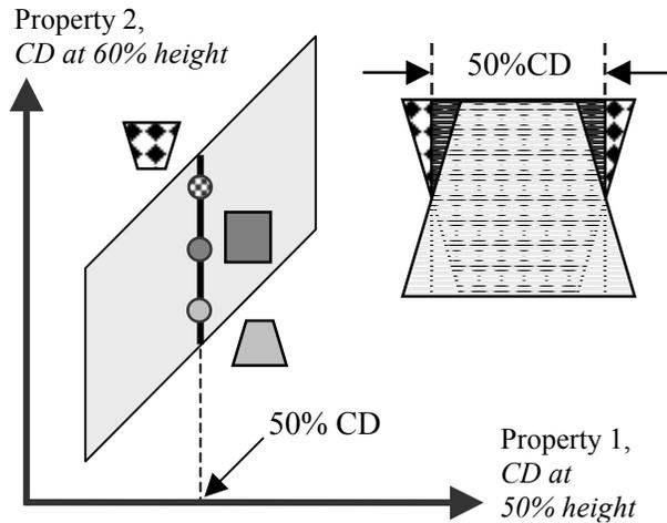
Figure 4. Comparison of two different sample properties: CD at 50% and at 60% height
