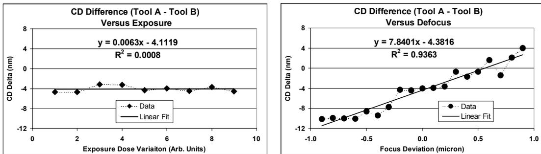
Figure 6. Differences of two CD-SEM tools versus variations in I-line resist FEM
