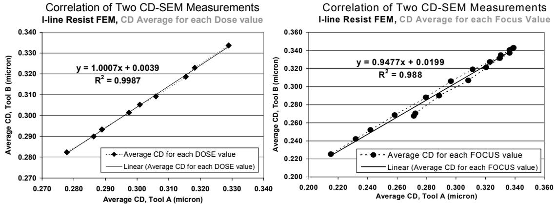
Figure 7. Correlation of two CD-SEM measurements
